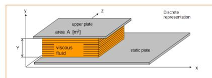
**Before instant t\_0** the fluid is contained between two large parallel plates of area A, separated by a very small distance Y
