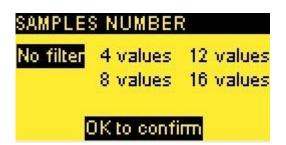
Sampling period: this period corresponds to the new viscosity value acquisition period. At each period, a new value enters in the table and the oldest is getting out. The filtered viscosity is updated.
