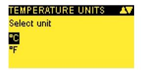
To choose the new temperature unit, it is enough to select it with the arrows and to press "OK". The change is automatically done.
