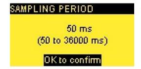
The first filtered viscosity value is calculated (samples number \* sampling period) after the starting of the sensor.
