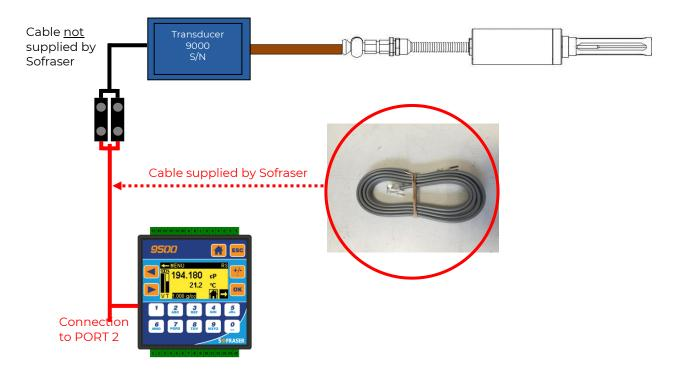
The 9510 electronic device has been designed in order to control 1 MIVI sensor. This means the MI-VI's transducer 9000 and the 9510 are connected in a RS-485 serial loop as shown in the scheme just above.
