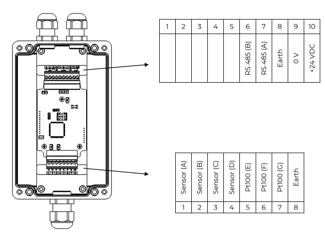
The wires at the end of the cable have the following allocations.
