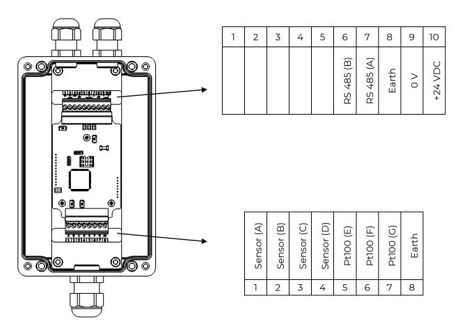
For standard MIVI cable, the wires at the end of the cable have the following allocations.
