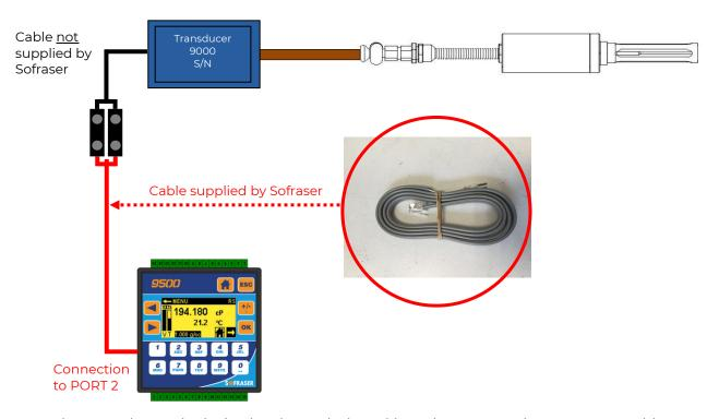
The 9510 electronic device has been designed in order to control 1 MIVI sensor. This means the MI-VI's transducer 9000 and the 9510 are connected in a RS-485 serial loop as shown in the scheme just above.
