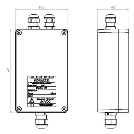
The processor must be connected to a stabilized and filtered **24 VDC** (± 2.4 VDC), 1 A power supply. The polarity of the power supply is highly important, in order to avoid any damage on the electronic board.
