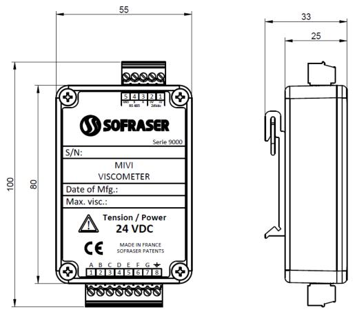
The processor must be connected to a stabilized and filtered **24 VDC** (± 2.4 VDC) power supply. The polarity of the power supply is highly important, in order to avoid any damage on the electronic board.
