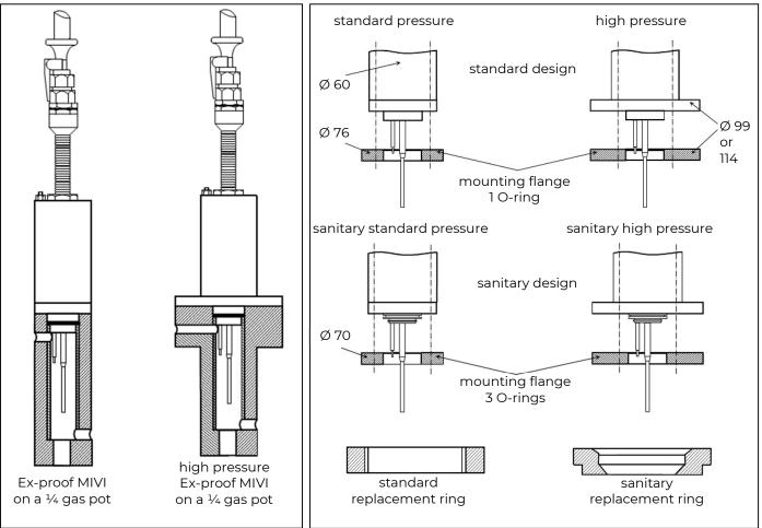
Details about mounting accessories are available in technical leaflets reference 320, 328 and 329 (see APPENDIX D). When it normal production cycle, the vibrating rod must be continuously and fully immersed in the fluid.
