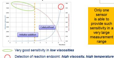
Only one sensor is able to provide such sensitivity in a very large measurement range
