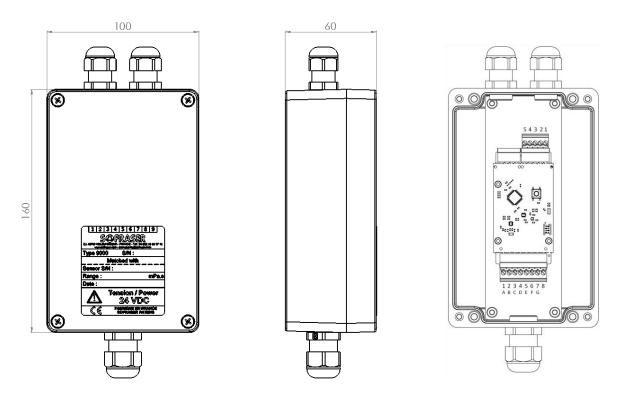
All the connections to the electronic device are made on the two terminal blocks located inside the enclosure. See chapter 2.3.1 for the wiring instructions.
