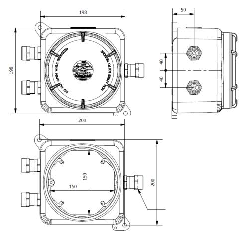
When installed in an ATEX enclosure, the 9000 transducer is in its standard IP20 enclosure. The terminal blocks are therefore identical to the ones described in § 2.2.1. See chapter 2.3.1 for the wiring instructions.
