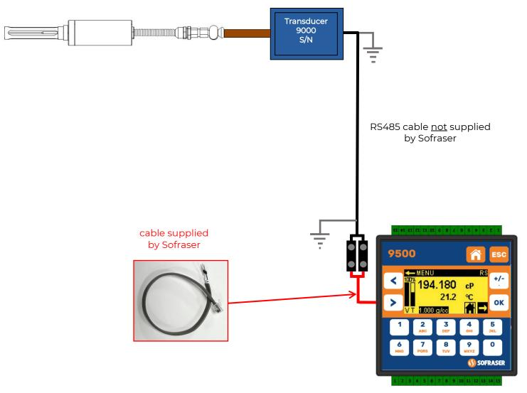
The internal termination resistance of the 9510 is activated. Check that the termination resistance at the end of the RS485 loop, on the 9000 transducer, is also activated.
